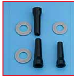
Right: Swollen seals caused by incorrectly applied instrument oil. Left: New seals
