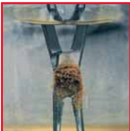
Corrosion caused by immersion in physiological salt solution over a period of several hours
