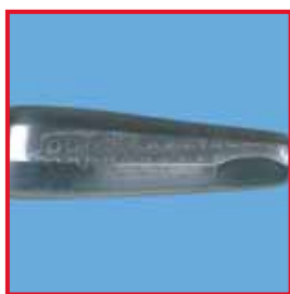
Carry-over of cleaning agent residues due to insufficient rinsing
