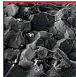
Detail: Jaw clamp with typical grainy, intercrystalline fractured structure.
