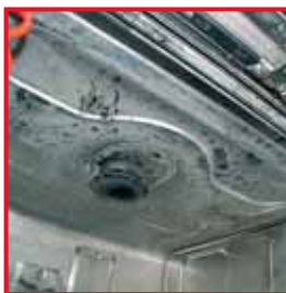
Rinsing chamber with heavy lime scale deposits
