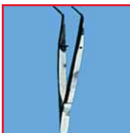
Partial etching effect and deposits of an etching agent causing hemostasis on the surface of the instrument. Cause: contact time too long
