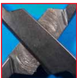
Corrosion due to insufficient use of care products
