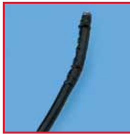
Swollen insertion tube caused by using unsuitable care agent.
