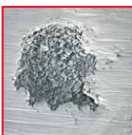
Pitting - seen under a scanning electron microscope - magnified 200 times
