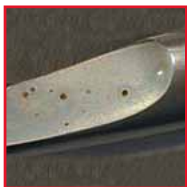
Pitting induced by chlorides on instrument.
