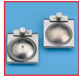
Right: Leaking flap valve on a trocar caused by the seal swelling as a consequence of contact with oil. Left: New flap valve
