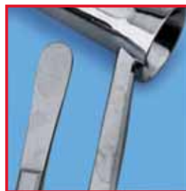
Consequence: Instruments with limescale residues
