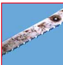
Material affected at partially defective chrome coating. Cause: Humidity causes corrosion to form on unprotected carrier material (normal steel)
