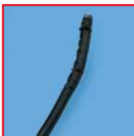
Swelling at distal end of fiberscope
