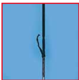
Damaged insulation on HF instrument
