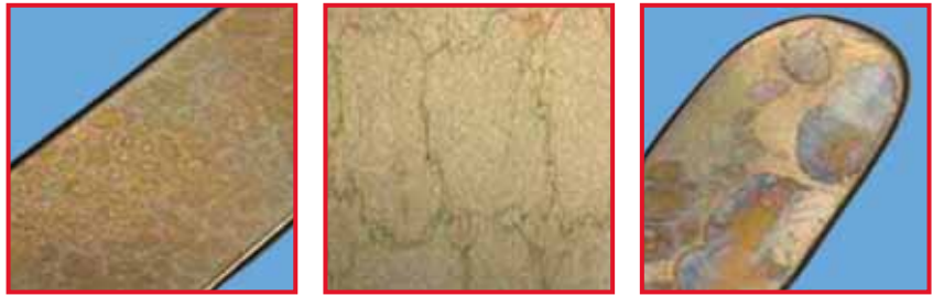
Typical silicate discoloration on the surface of the instrument after steam sterilization caused by excessive silicon dioxide levels in the demineralized water.
