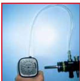
Manual leakage test on flexible endoscope
