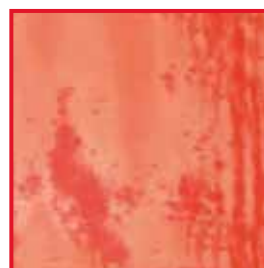
Material affected on natural/colored anodized aluminum surface of containers. Cause: alkaline washer solution above permitted level
