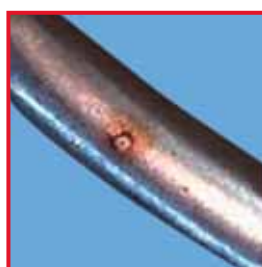
Pitting on tweezers. Cause: Over-aging of color-coding band allows harmful substances containing chloride to infiltrate.
