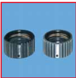
Image page right: Corrosion of black anodized instrument surfaces by softened water.
