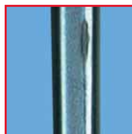
Contact corrosion: Stainless steel/Brass
