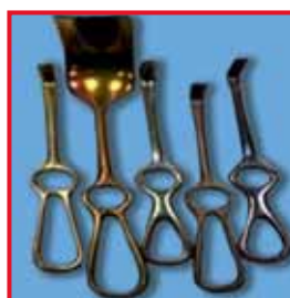
Typical silicate discoloration in the washer-disinfector chamber and on the surface of the instrument caused by a detergent containing silicate, or excessive levels of silicon dioxide in the water.
