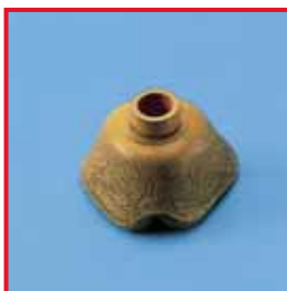
Aging tears in a breathing mask
