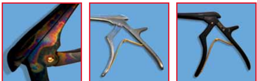
Example: black, TiAlN coated punch. Inside colors, or coat complete removed with undamaged, gilded components (end screw, springs).
