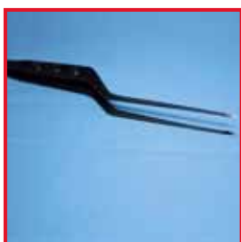
Deformation caused by improper handling
