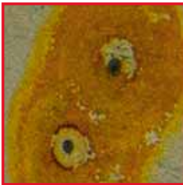
Reactivation salt containing chloride caused massive pitting on the surface of the instrument. Leaking ion-exchanger connection in the W/D.
