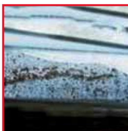
Partial etching effect and deposits of an etching agent causing hemostasis on the surface of the instrument. Cause: contact time too long
