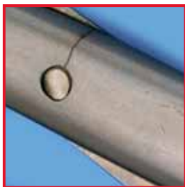
Stress cracks next to scissor hinge
