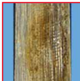
Bone punch, friction surface on sliding section indicates onset of friction corrosion.
