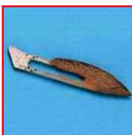
Surface of blade affected due to humidity. Cause: Composition of materials, normal steel, so disposable product.
