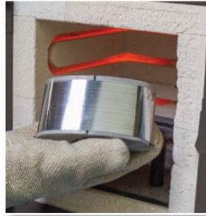
Heat-treatment sets the archform shape to wire.
