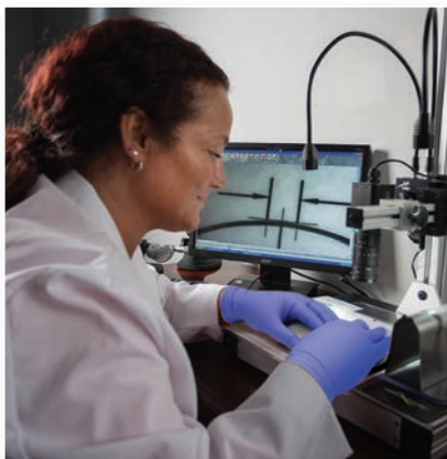
G&H employee, Laura – All archwires are evaluated for consistency of shape.
