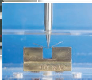
3-point bend testing.
